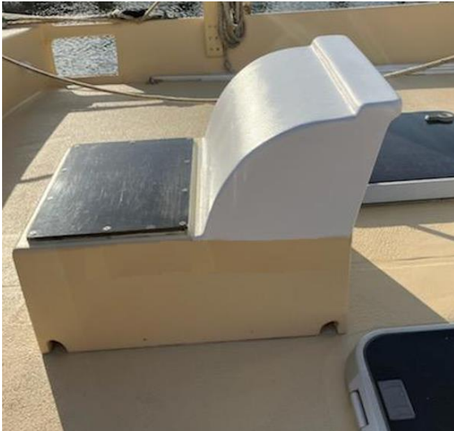
Photo 13 – Dorade with skylight ( back )
