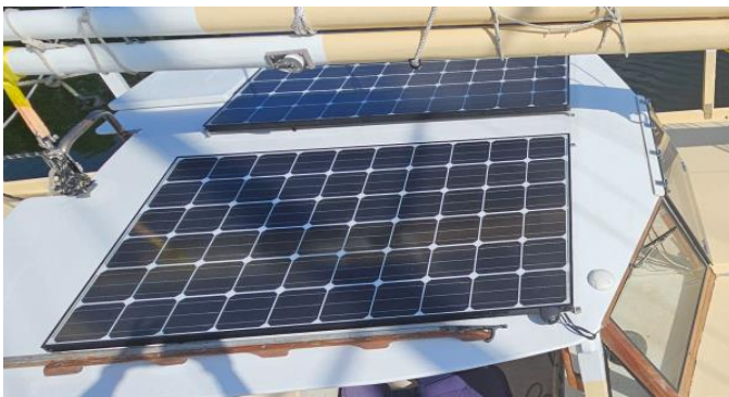
Photo 15 – Solar panels on hard dodger ( back )
